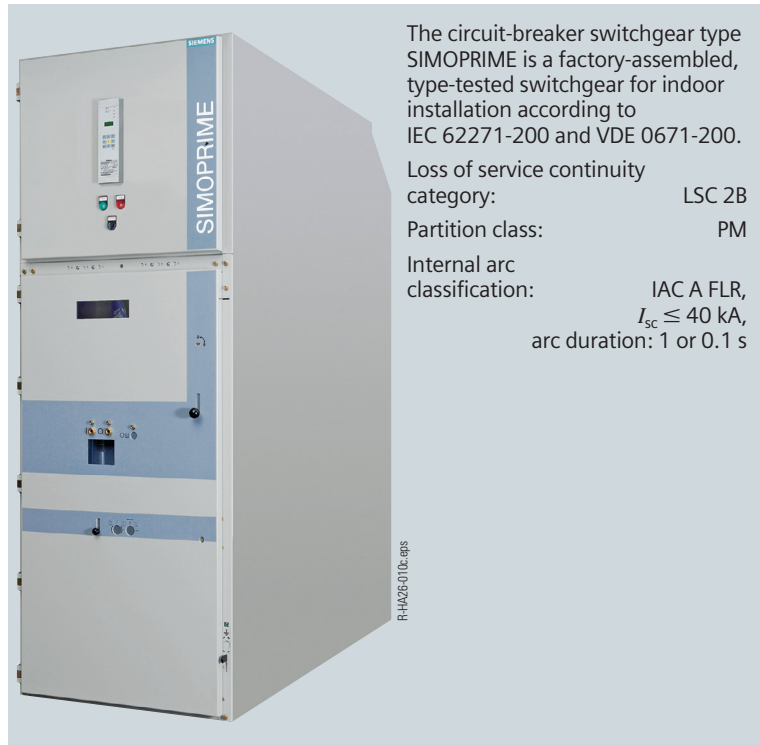
SIMOPRIME panel Maximum ratings 17.5 kV / 40 kA / 3600 A
